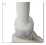
5.Use the frit insertion rod to press the frit into place.
