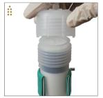
7.Replace the screw cap on the cartridge.
