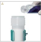
3.Add media into the headspace of SL cartridge, and tap the SL cartridge lightly on lab bench to let the media settle. Do not overfill.
