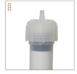
8. The tightening process will set the frit in place.
